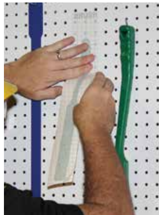
Use liner grid lines to align shadow on board. Peel off back liner and press shadow in place.
