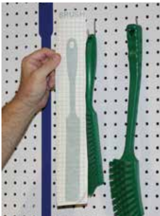
Precision die-cut adhesive vinyl shadow replicates size, shape, and color of the tool.
